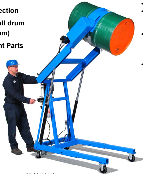
Model 410-110 with 72" (183 cm) dispensing height and electric power lift and tilt.
