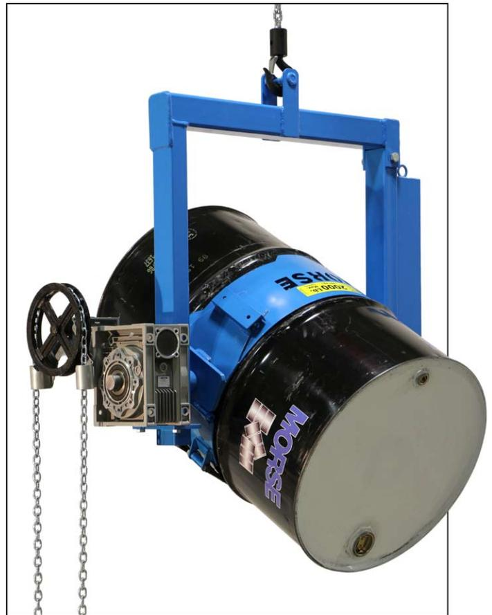
Manual drum tilt is controlled with a 12' (366 cm) pull chain loop hanging 6' (183 cm) below the chain wheel. There is enough resistance in the enclosed gear box to automatically stop and hold the drum tilt angle. Hand wheel tilt control option is also available.
