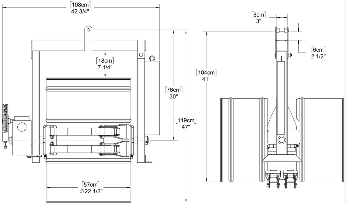
NOTE: Standard loop of pull chain extends approximately 6 feet (1.83 m) below the chain wheel.
