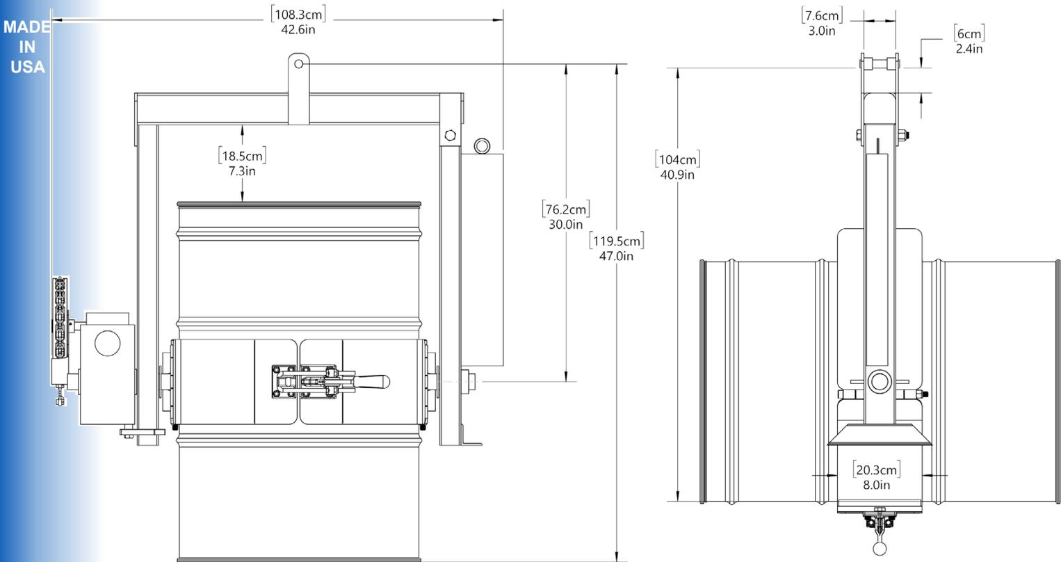
NOTE: Standard loop of pull chain extends approximately 6 feet (1.8 m) below the chain wheel
