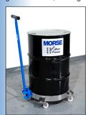
The Clamp+GO™ can be used with round drum dollies of various sizes. Move the quickpin to adjust for 2", 2.5" or 3" (5.08, 6.35 or 7.62 cm) tall dolly sidewall. Clamp+GO™ works with all Morse round drum dollies, and with many other brands.
