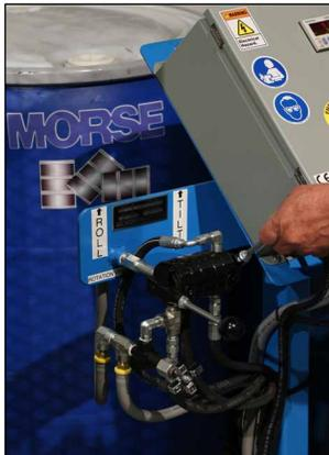
7. Use TILT handle to raise the drum into rotating position
