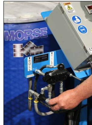
9. Adjust drum rotation from 4 to 16 RPM
