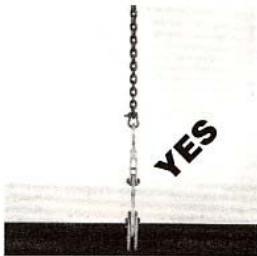
Photograph C Sing directly above and in line with shackle.
