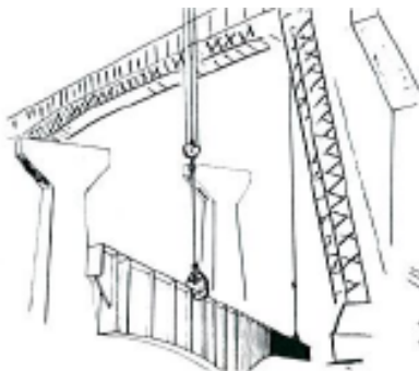
Two model SEA's can be used for handling exceptionally long beams or girders.
