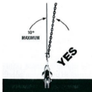
Photograph D Maximum allowable sideloading.
