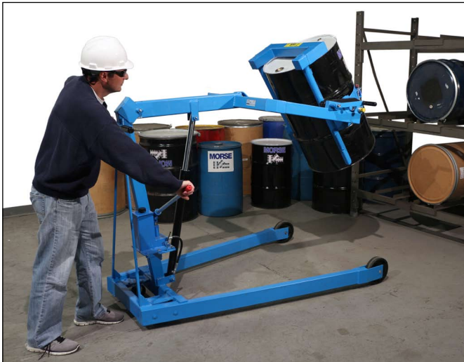
Raise drum and rotate to horizontal drum racking position.
