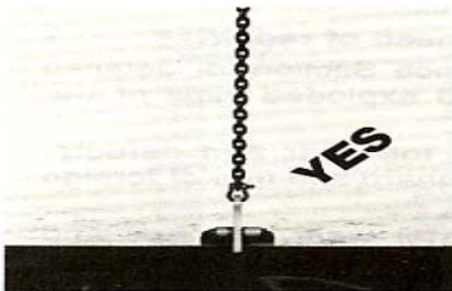
Photograph G Sling directly above and in line with cam.
