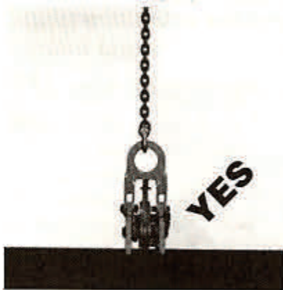
Photograph J Sling directly above and in line with the lifting shackle.
