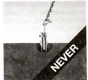
Photograph E Excessive side loading.
