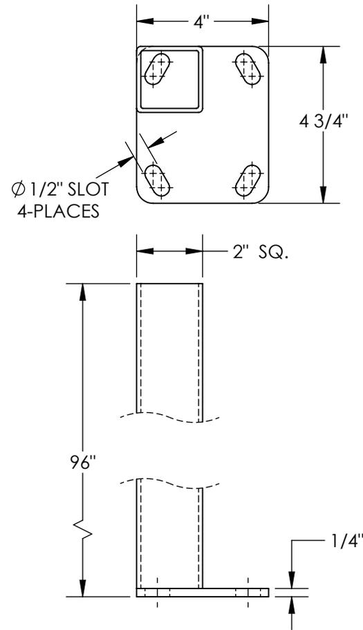
APG KIT #23-154-014 CONTAINS THE BRACKETS AND HARDWARE FOR MOUNTING THE APG-M PANELS. THERE ARE (4) KITS INCLUDED WITH EACH PANEL. THE BRACKETS ARE ATTACHED TO THESE POSTS WITH SELF-DRILLING SCREWS INCLUDED IN THE APG KIT. THE SCREWS ARE LOCATED DURING ASSEMBLY BY THE CUSTOMER TO ALLOW CUSTOM PLACEMENT.
