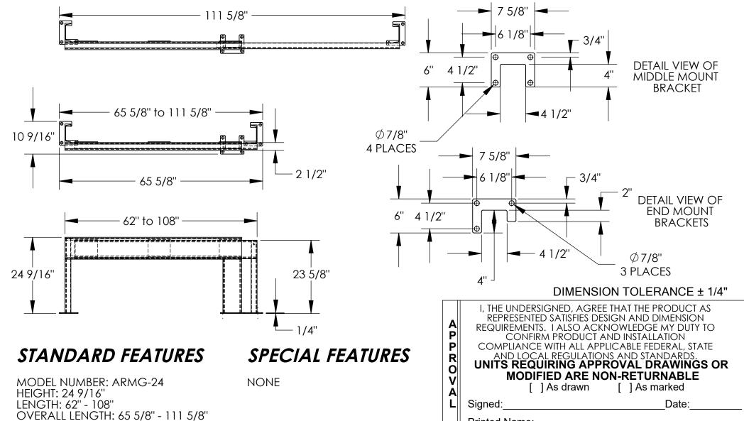
FRAME: STRUCTURAL C-CHANNEL BASE PLATES: 7 5/8" X 6" X 1/4"
