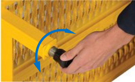
Turn leg counterclockwise to increase platform height
