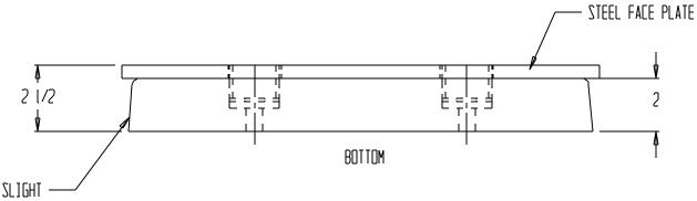
NOTE: OVERALL DIMENSIONS & HOLE CENTERS TAKEN FROM BOTTOM OF BUMPER
