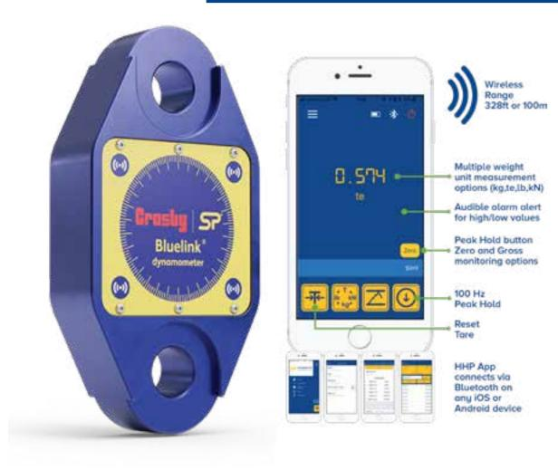
Designed to replace outdated mechanical products still in the field, this 14,300lb (6500kg) Dynamometer, the 'BlueLink', is the latest Crosby SP product to feature their proprietary Bluetooth wireless technology.
