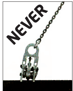
Excessive side loading.
