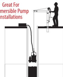
The listed load rating reflects the davit crane boom position as well as manual winch operation, assuming average lifting effort. Handle effort will increase as the cable is spooled onto the drum. Load rating and ease of lifting depend on the boom position, specific winch style, and the user's lifting effort. Dimensions and illustrations are for reference only and subject to change without notice.
