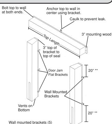
Bolt on leg of the bracket to building Bolt other leg to side of dock seal using the two lad bolts provided.
