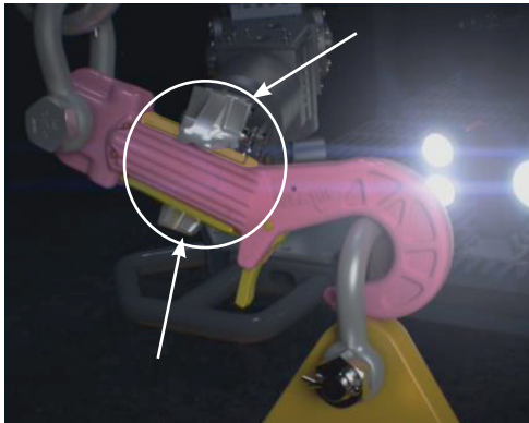
Pic. 5: Press the release/locking and the securing latch
