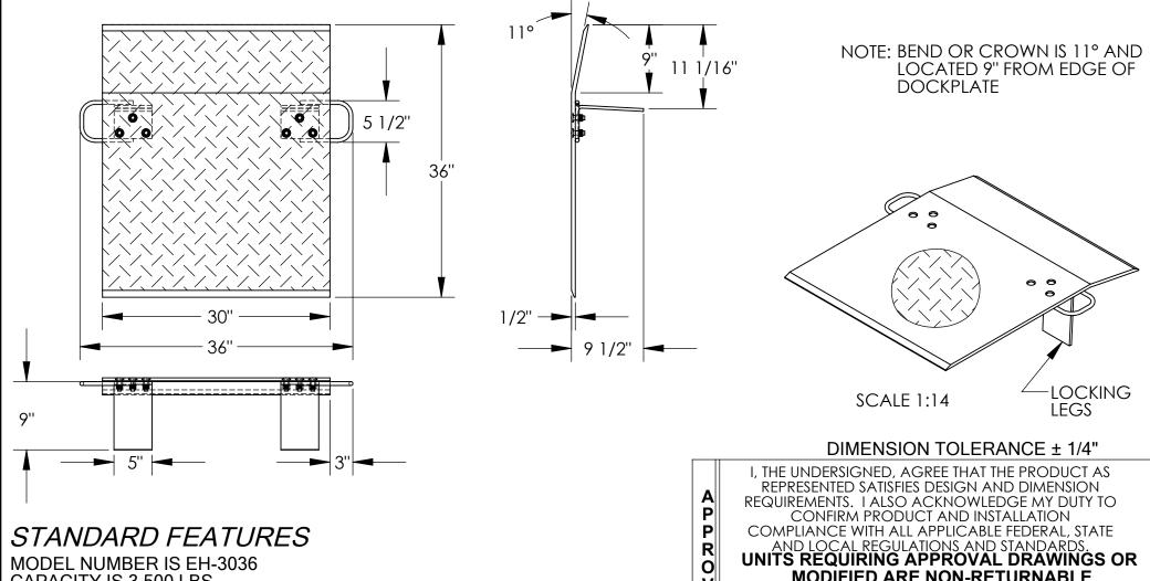
CAPACITY IS 3,500 LBS. **OVERALL WIDTH IS 36" DECK WIDTH IS 30" OVERALL LENGTH IS 36" OVERALL HEIGHT IS 9 1/2"** THICKNESS IS 1/2" HANDLES ARE 5 1/2" x 3" LOCKING LEGS ARE 5" x 9"
