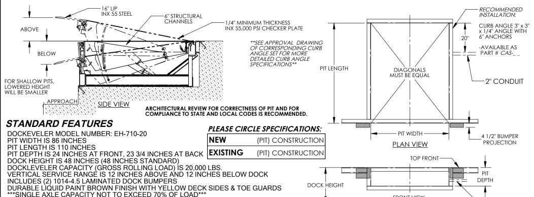
ALL STRUCTURAL STEEL CONSTRUCTION WELDING MEETS AWS.
