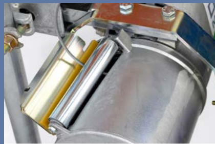
Automatic slack rope switchdrive is shut down when the wire rope gets loose
