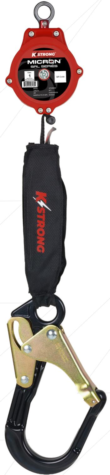
The Micron™ series of SRL's have not only been tested to ANSI Z359.14-2021 but also to a Fall Factor of 2. This means that when a preferred overhead anchor point is not present, a worker may connect to a suitable anchor up to 5 ft. below the dorsal D-ring height of their full body harness.
