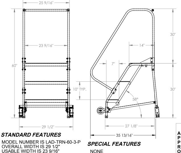
MODEL NUMBER IS LAD-TRN-60-3-P **OVERALL WIDTH IS 29 1/2"** USABLE WIDTH IS 23 9/16" **OVERALL LENGTH IS 35 13/16" USABLE LENGTH IS 27 1/8" OVERALL HEIGHT IS 60"** PLATFORM HEIGHT IS 30" **COLOR IS VESTIL BLUE** STEP TYPE IS PERFORATED CLIMB ANGLE IS 58° STEP DIMENSION IS 24" x 7" TOP STEP DIMENSION IS 24" x 14" MAX CAPACITY IS 350 LBS
