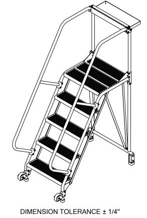
MODEL NUMBER IS LAD-TRS-60-5-P **OVERALL WIDTH IS 29 1/2"** USABLE WIDTH IS 23 9/16" **OVERALL LENGTH** W/ TOOL TRAY IS 62" **USABLE LENGTH IS 46 3/8" OVERALL HEIGHT IS 80"** PLATFORM HEIGHT IS 50" **COLOR IS VESTIL BLUE** STEP TYPE IS PERFORATED CLIMB ANGLE IS 58° STEP DIMENSION IS 24" x 7" TOP STEP DIMENSION IS 24" x 21" MAX CAPACITY IS 350 LBS
