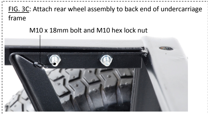
FIG. 3A: Attach steering assembly (M) and rear wheel assembly to undercarriage frame
