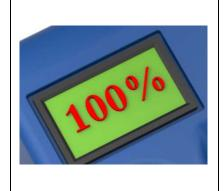
1) 100% fully charged battery 2) 20% battery is low and needs to be charged immidiately or replaced with another fully charged battery 3) 10% charge will support maximum of 40 - 50 steps before unit turns off.
