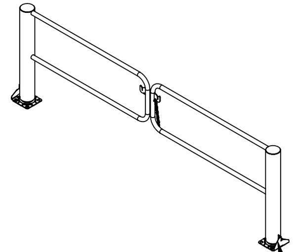
STOP BRACKETS MOUNT ON INNER POST BASES TO CONTACT STOP TABS ON BOTTOM OF OUTER POSTS
