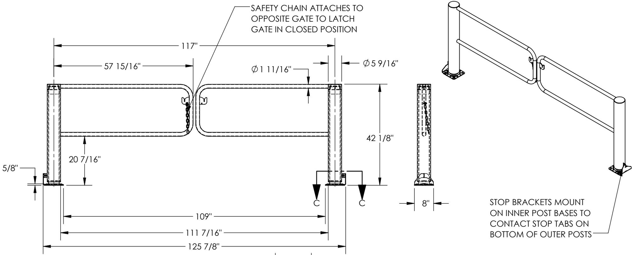
STOP BRACKETS MOUNT ON INNER POST BASES TO CONTACT STOP TABS ON BOTTOM OF OUTER POSTS
