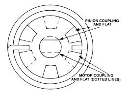
Figure 6-1B. Brake Spring, Motor and Pinion Coupling Alignment
