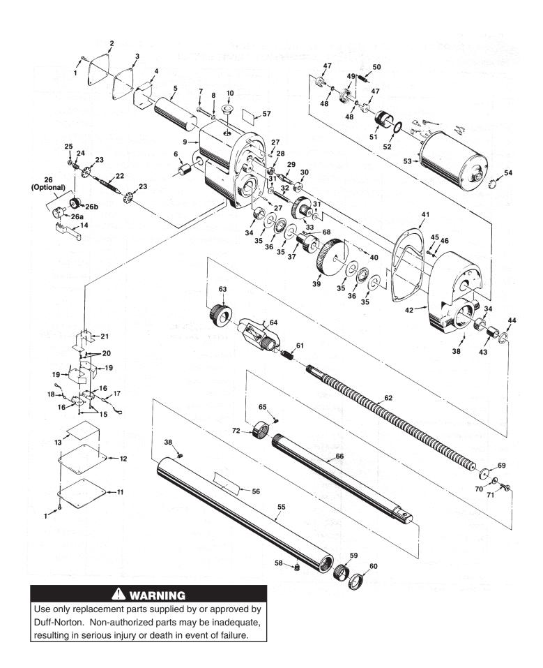
Figure 5-1. Exploded Parts Illustration 6420 & 7420 Series AC Ball Screw Actuator
