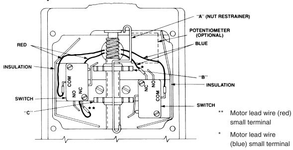
Figure 6-3. Limit Switch Assembly, 6420 & 7420 Series AC Ball Screw Actuator
