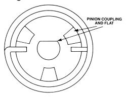
Figure 6-1A. Brake, Spring, Motor and Pinion Coupling Alignment
