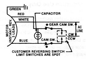
Figure 1-2. Limit Switch Wire Color Diagram
