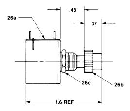
Figure 4-1. Potentiometer Nut and Washer Assembly
