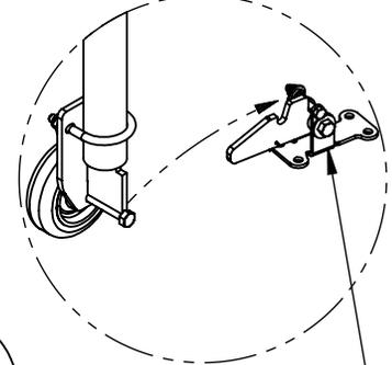
LATCH MAY BE ROTATED 180° TO ALLOW GATE OPENING IN OPP. DIRECTION
