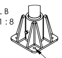
Ø3/8" HOLES FOR MOUNTING HINGE TO FLOOR (4-PLACES)
