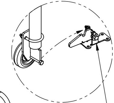
LATCH MAY BE ROTATED 180° TO ALLOW GATE OPENING IN OPP. DIRECTION
