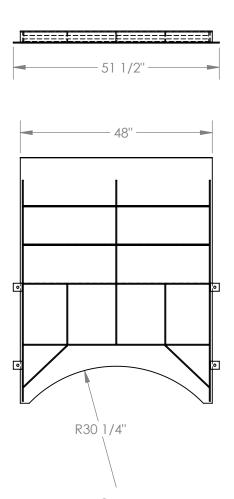
STANDARD FEATURES MODEL NUMBER IS SWA-R-60-AW **OVERALL LENGTH IS 61 13/32" OVERALL HEIGHT IS 3" OVERALL WIDTH IS 51 1/2" USABLE WIDTH IS 48"** MAX CAPACITY IS 4,000 LBS.
