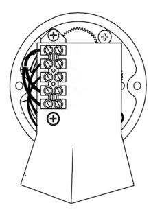
Figure 2-2. Terminal Block Connections (AC)
