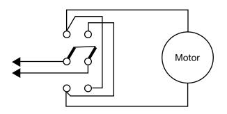
Figure 2-3. Wiring Schematic DC with Clutch
