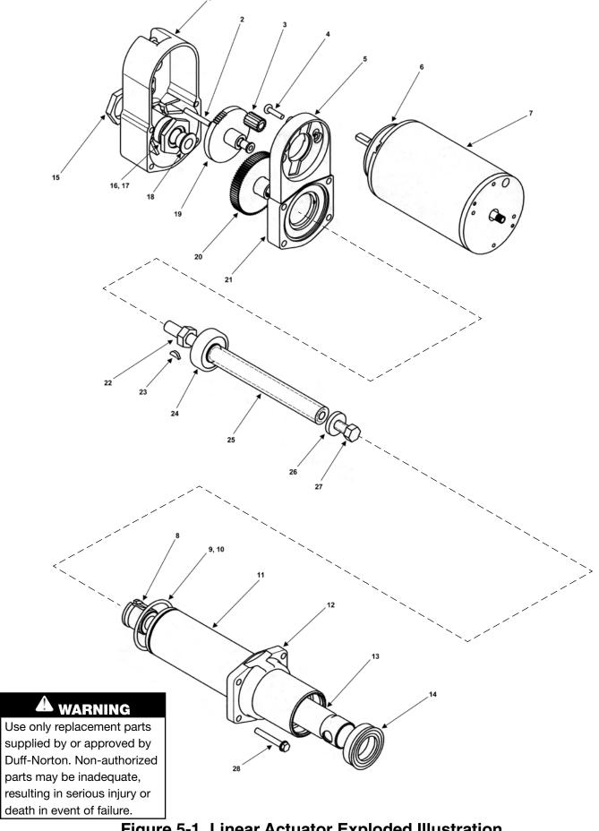
Figure 5-1. Linear Actuator Exploded Illustration
