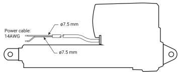
Figure 2-4-1. Cable Without Signal
