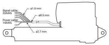
Figure 2-4-2. Cable With Signal
