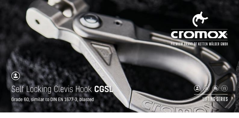
Load hooks are an essential component in the use of chain slings and assemblies, contributing significantly to the stability and safety of the lifting process. The automated closing mechanism ensures secure fastening when loaded, enhancing operational safety. The bionic design allows for a high working load limit (WLL) while reducing the weight. The advantage of the clevis hook is that no additional connecting links are required as the chain can be hooked in directly.
