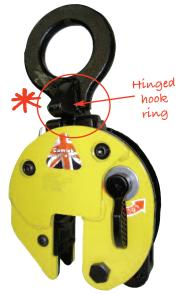
The CY plate clamps with hinged hook rings can be used for the safe handling of plate at various angles. It can lift plate from the horizontal and put it down in the vertical. The hinged hook ring ensures adequate gripping pressure in every position, but the load capacity reduces. See the diagram below showing the load / force capacities.
