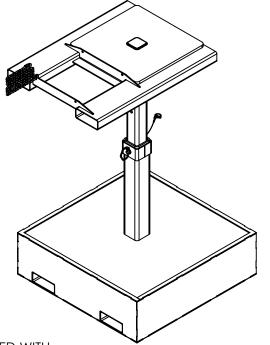
NOTE: UNIT IS FILLED WITH **GRAVEL OR LIMESTONE** AGGREGATE CONCRETE.
