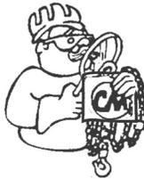
Check for gouged, twisted, distorted links and foreign material. Do not operate hoists with twisted, kinked, or damaged chain links.
