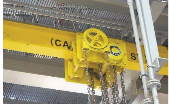
SPARK RESISTANT/EXPLOSION PROOF, 5-TON CHESTER ZEPHYR LOW-HEADROOM TROLLEY HOIST IN USE ON AN OFFSHORE OIL PLATFORM.
