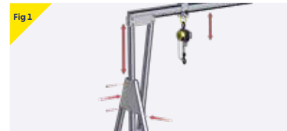
Beam height adjustment bolts (2 bolts on each upright). Tighten all bolts to 27 Nm (20 ft lbs) or until spring washers are fully depressed.
