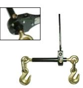
Color marking: Green WLL: 13,000 lb Chain size: 1/2"-5/8" Proof tested to: 19,500 lb Safety factor: 3:1 Common applications: Equipment transport Heavy hauling Steel coil transport
