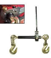
Color marking: Red WLL: 9,200 lb Chain size: 3/8"-1/2" Proof tested to: 13,800 lb Safety factor: 3:1 Common applications: Equipment transport Heavy towing Steel coil transport
